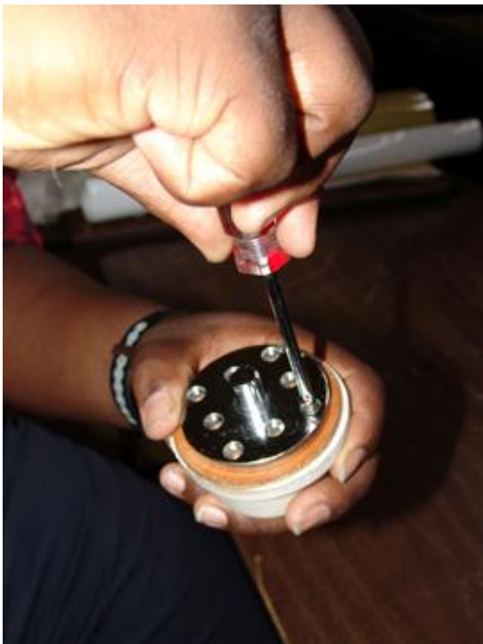
Screw the Pad to the Pad Holder.
